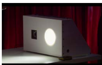
Fig 3: Li-Fi Transmission using LEDs
